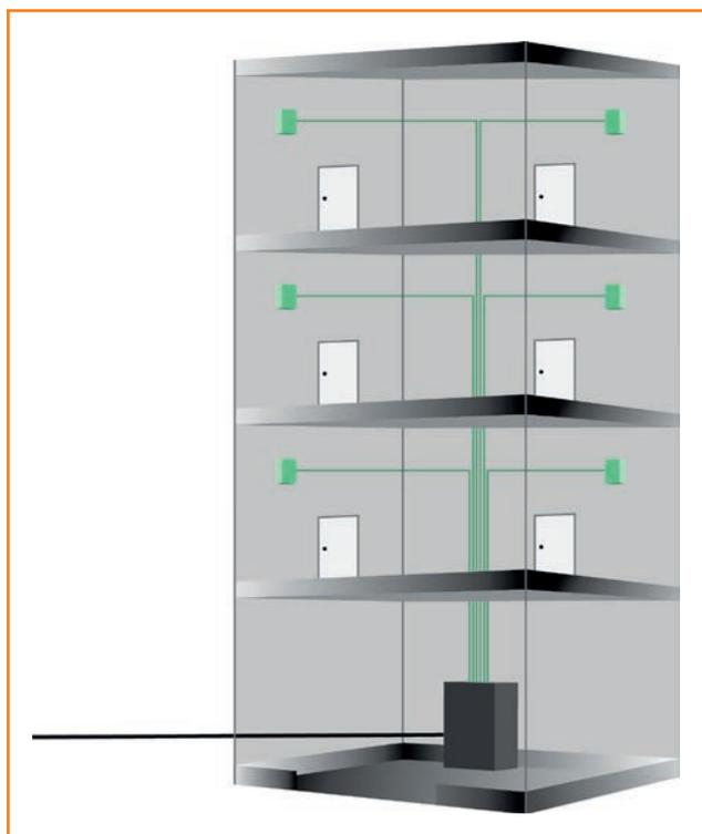
**Figure 1: Multi-fibre riser**
