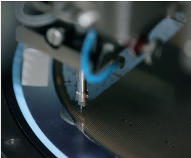
Wafer – GaAs Die being picked from Wafer for eutectic die bonding to carriers.
