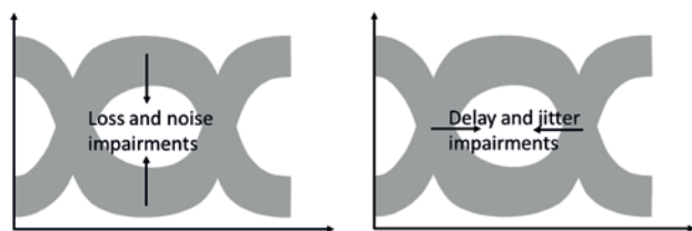
Figure 12: Illustration of eye closure due to Loss and noise (left) and delay and jitter (right).
