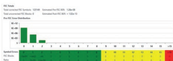
Figure 21: Example of BER histogram (from XENA Networks ... manual).
