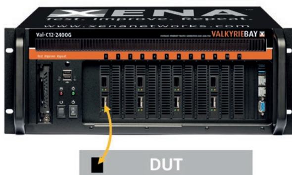
Figure 19: Example of test set-up for single port testing.
