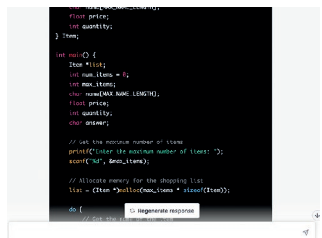
Figure 3: Some 'c' code generated by ChatGPT. Note that max_items could be any int value, potentially allowing a very large value to be given.
